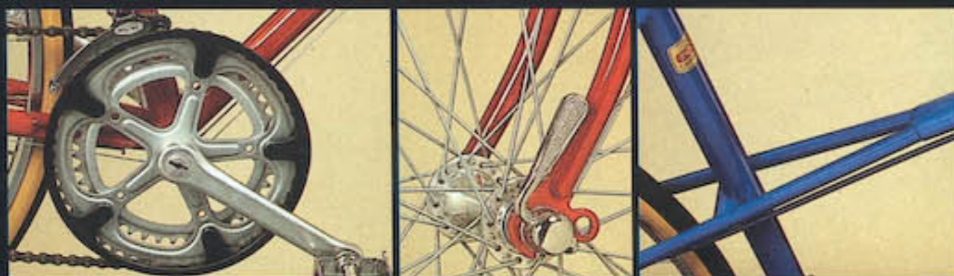
1 - PROFILED COTTERLESS ALLOY CRANK. - 2 - ALLOY QUICK RELEASE HUB. - 3 - MOTOBECANE UNIQUE MIXTE DESIGN.
