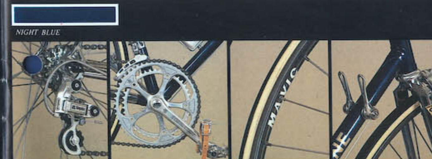
1 - MOTOBECANE SIMPLEX DERAILLEUR AND REAR CHROMED STAYS BASES. — 2 - STRONGLIGHT CHAINWHEEL WITH MAILLARD 700 PEDALS AND CHRISTOPHE TOE CLIPS. — 3 - MAVIC SSC RIMS. — 4 - COLUMBUS FORK WITH CINELLI CROWN.
