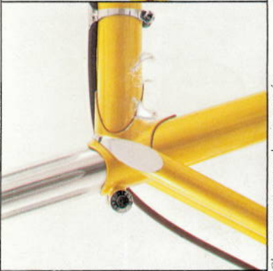
Chrome wrap-around seat stays for strength. Brazed-on seat binder lug with chromoly dual allen head binder bolt for positive locking.
