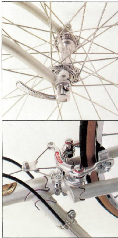
Suzue quick release alloy small flange hub. Lightweight, less friction. Forged fork ends for strength.
