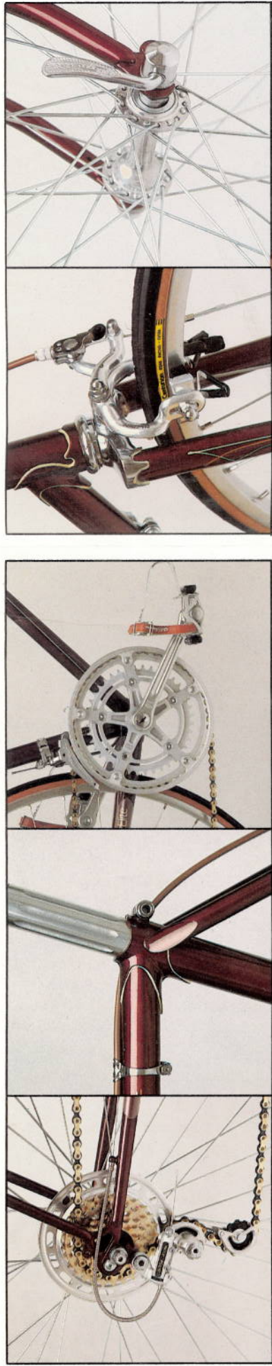
Suntour Cyclone GT Derailleur system with Suntour Train-Z cluster and chain. Inner edges of chain's outer link plate are deeply scalloped; so chain operates at a sharper angle, engaging cluster teeth more quickly for greater shifting speed.
