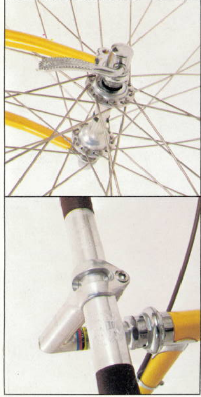
Sunshine Pro-Am small flange, quick release hubs with precision ground races for minimal friction. Stainless steel spokes.
