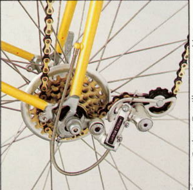
Suntour Cyclone Derailleur system. Most advanced system available. Unique slant parallelogram mechanism enables pulleys to shift diagonally at same angle as sprocket during gear change, retaining uniform clearance between pulleys and sprocket. Result: More stable driving, easier shifting. Suntour's new Tran-Z chain and Tran-Z cluster dramatically improve shifting speed.
