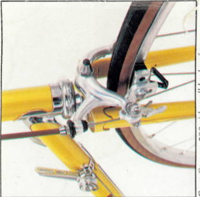
Gran Compe 500 side pull brakes for positive response, all-weather braking action. Chrome sloping fork crown, chrome head lug add style. 700c 19.6mm wide alloy rims and 700c Centurion 25mm 100 psi skin tires, for racing performance.
