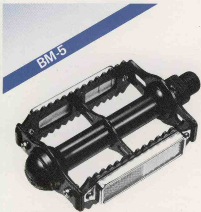
No. 2507 Motorcross, made of steel, w/Cr. Mo. steel spindle Winged dust cap Gold, red, blue, black & c-p color available. Size: 82 mm. Weight: 540 grm. (CPSC/CHP/AS approved)
